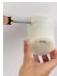
2. Set timing and light level and plug in connections
