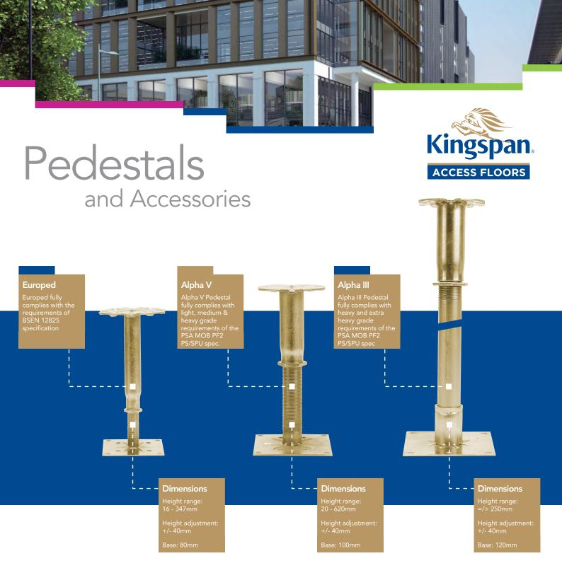
The pedestals are of a Zinc plated steel construction, ensuring electrical continuity, pre-assembled to help minimize installation time. The pedestals have a locking nut to ensure that once adjusted and locked there is no movement in the pedestal head.
